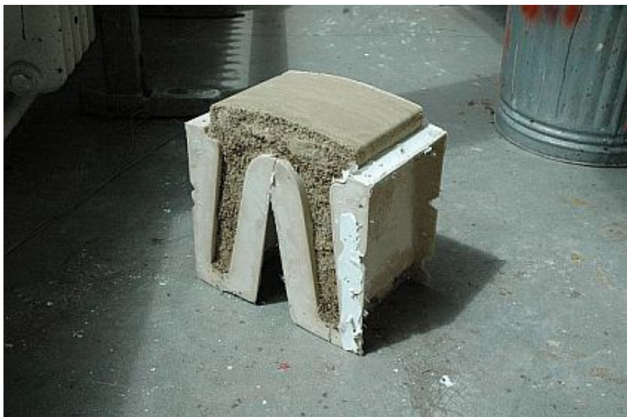
Stool being removed from its mould by Damian Palin
