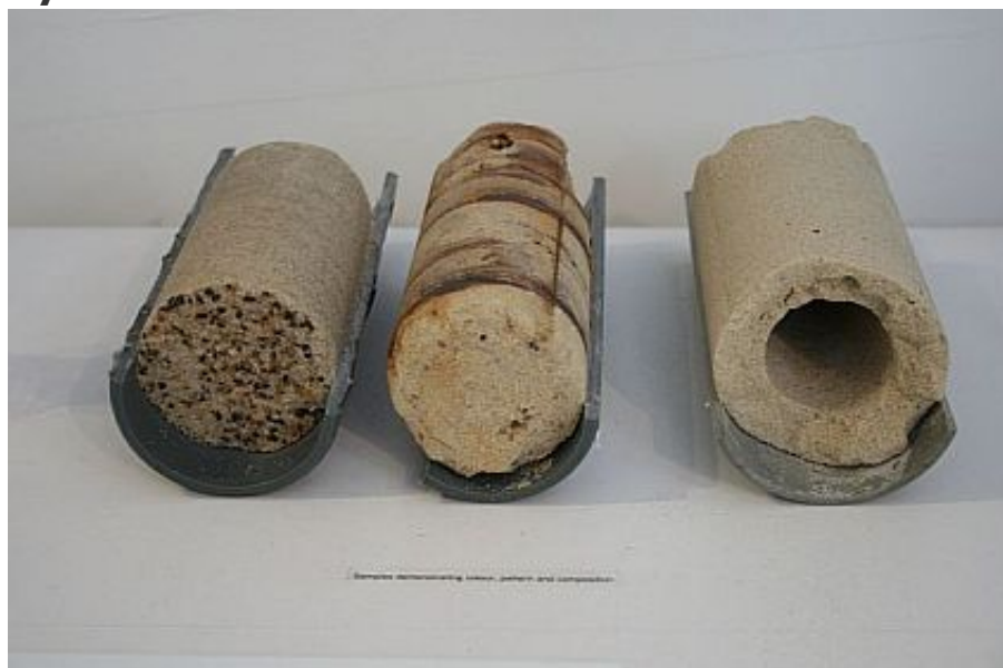
Synthetic stone samples by Damian Palin
